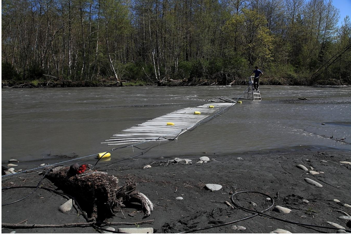
Figure 2. Photo of the HRC DIDSON site showing the picket weir and the ladder on which the DIDSON is mounted.
